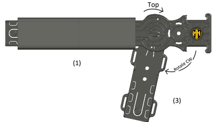
**Step 1 (Cont.)** Insert screws (9) through Mounting Rail (1) as shown.
