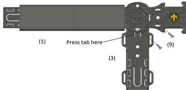
To disassemble reverse the process while depressing the bottom screw tab when rotating Support Strut (3).
