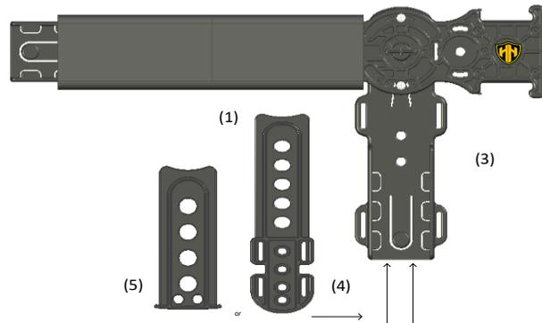
**STEP 2:** Support Strut (3) comes attached with Short Base (5) for imports, sports cars, and most sedans. Attach the Long Base (4) into the Support Strut to the desired seat height (9"-12") from floor board (Trucks and SUV's).
