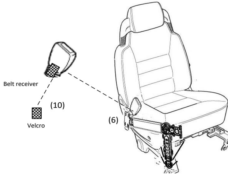
**STEP 5:** Apply a Velcro strip (10) to the backside of the seat belt receiver as shown. Slide Multi-Mount into the gap space between the seat(s) or console. It may require to start with Multi-Mount from front of seat and work backwards into gap. Some effort is necessary to get Multi-Mount into position to obtain a snug fit. Wrap 8" Cinch Straps (6) around the seat belt receiver (comes attached to Strap Mount).
